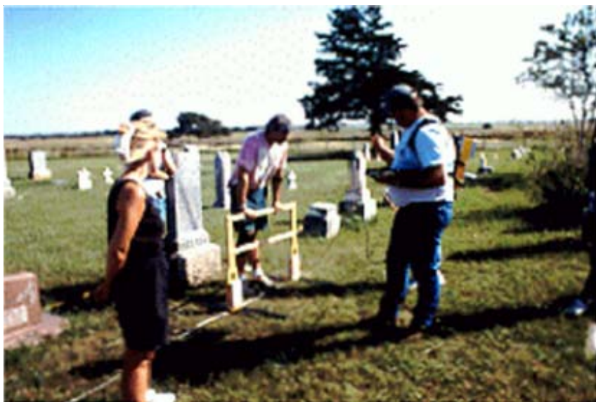
Figure 8. Use of a magnetometer to locate unmarked graves in a historic cemetery.
