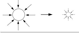
This phenomenon is called CAVITATION and it -Reduces capacity -Damages the pump
