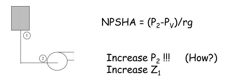
This is the reason why pumping fluids that are close to saturated conditions require that the vessel upstream be elevated. Flash tanks are typical examples of this.
