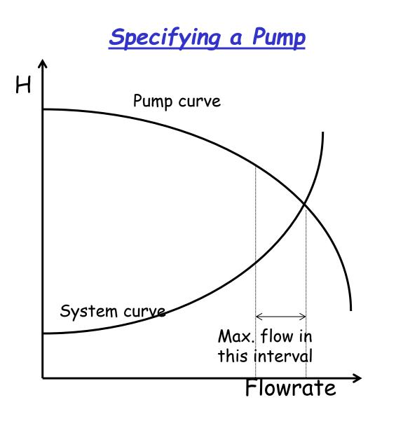
Since Hs = Hp , pick the Hs curve close to 80% open, at maximum flow What to do if NPSHA is too low
