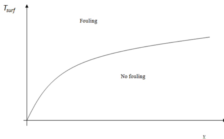
Figure 1. Representation of the threshold concept in relation to the surface temperature ( T_{surf} ) and the flow velocity ( v ).
