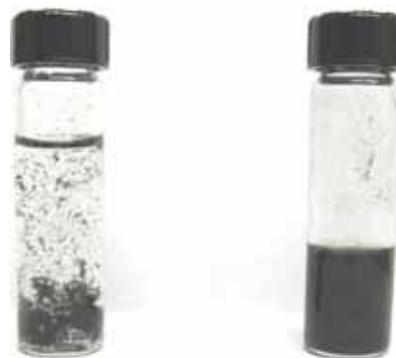
Figure 1. Comparison of SWNT suspensions. Left: no HRP protein was added and the suspension of SWNTs in sodium cholate was dialyzed for two days using a 10 kDa membrane. Right: SWNTs suspended in sodium cholate with HRP added were dialyzed, first with a 10 kDa membrane and then with a 100 kDa membrane. The SWNT-protein suspension was held at 4°C for ten days.
