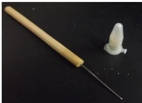
Figure 1. Dry yeast shaker (right), dissecting needle used to perforate the microcentrifuge tube (left), and five grains of yeast ejected by a single strong shake.
