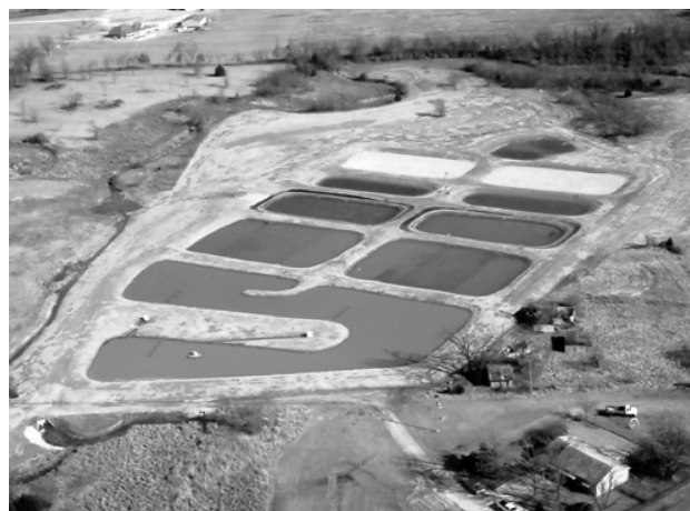
Aerial view of completed passive treatment center. Orange mine water flows from bottom of photo to clear water at the top.
