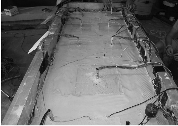
Centrifuge model is being instrumented
