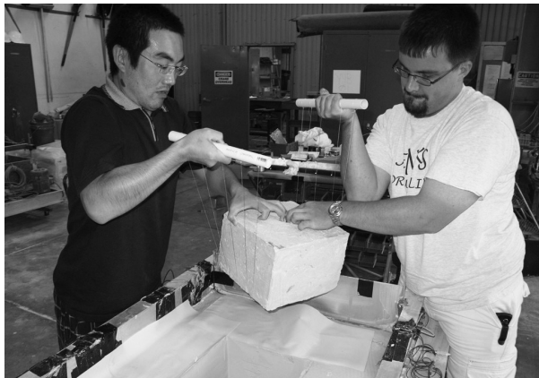
Liu and Price lowering a CDSM block into the centrifuge model
