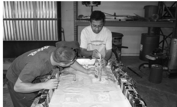
Muraleetharan and Thompson driving a centrifuge model pile
