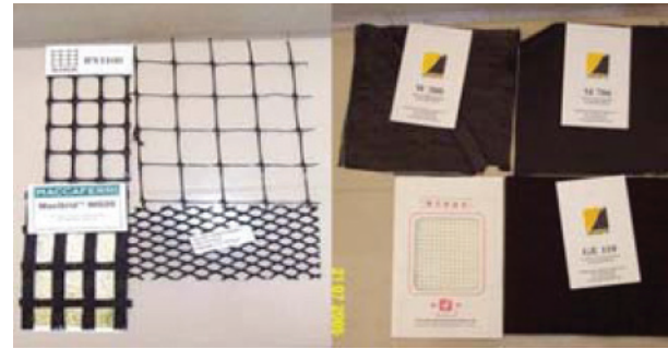
Figure 1. Geosynthetic samples: Geogrids, Geonet, Geotextiles, Geomembranes and Geosynthetic Clay Liners (GCL)
