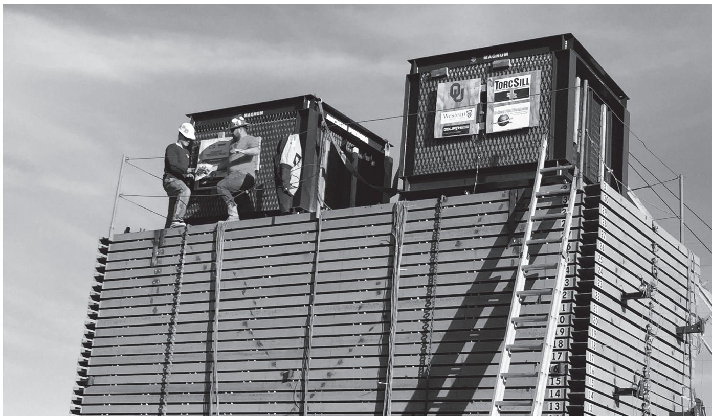
Shake Day 4 and 5 - The skids are loaded with sand to simulate fixed and pinned conditions.
