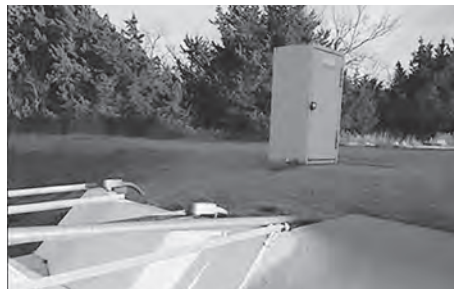
Control watershed test flume and sampling station; the gun safe houses the automatic sampler and related gear
