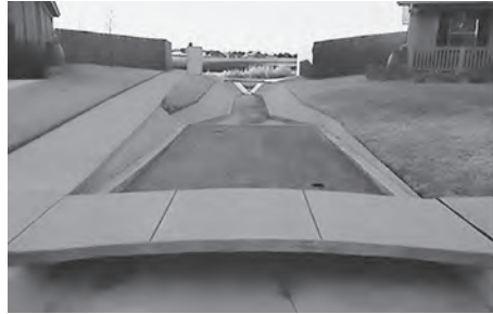
Treatment watershed test flume showing approach and permeable pavement section with sampling station in background; the gun safe houses the automatic sampler and related gear
