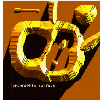
(b) Topographic analogy of the grayscale image
