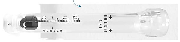
Hold the Depth Gauge ( $\mathbf{D}$ ) and insert the spinner with the NMR sample into the top of the Depth Gauge. Then push the NMR tube down gently while rotating until it ouches the black stopper surface of the Depth Gauge ( $\mathbf{D}$  and  $\mathbf{E}$ ).
