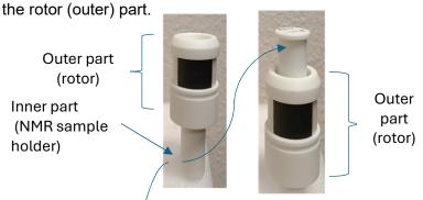
3. Make sure the inner part (holder) is <u>pulled down all the way</u> before inserting the sample into the spinner.
