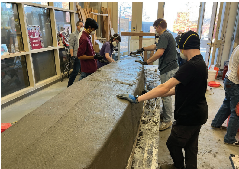
Concrete Canoe being fabricated in the Engineering Practice Facility. This student competition team designs, builds and tests a canoe made completely out of concrete and supports student rowers.
