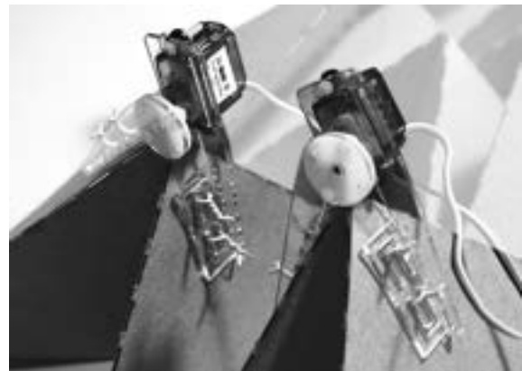
Figure 3. Detail of servo and mounting fixture. There is no structural skeleton; the actuation system is a distributed network with each unit mounted to the surface.
