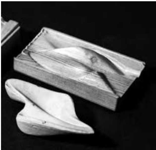
Fig. 3. A close-up photograph of the smallest iteration. Note the air bubbles on the sides of the unit due to the orientation of the pour. Photographs provided by Hengchen Liu.
