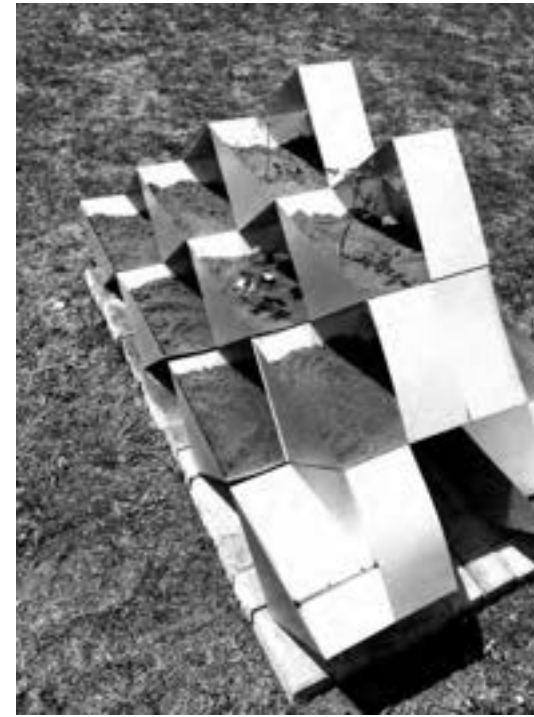
Fig. 3. Vertical Garden prototype. 24ga. Galvalume and steel rivets. Students: Aaron Ellzey, Jared Robinson, and Samuel Vick.
