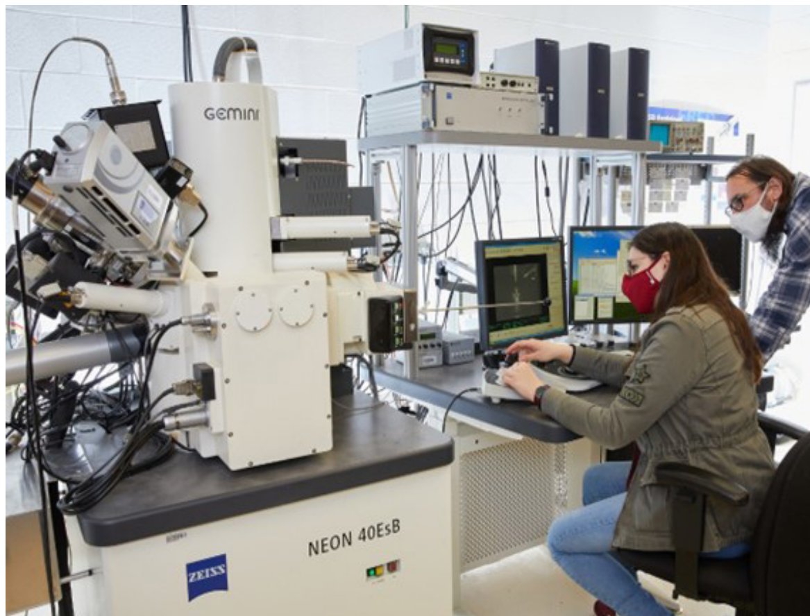
Above: Preston Larson from SRNML working with a physics student on the dual-beam FIB-SEM
