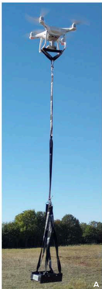
Figure 1 – A: The complete setup of the magnetic survey installed on a small drone (The non-metallic sleeve carries the smartphone which is mounted below the drone with a 1.5 m non-magnetic cable). B and C: Operating the drone. D: the exposed wellhead.
