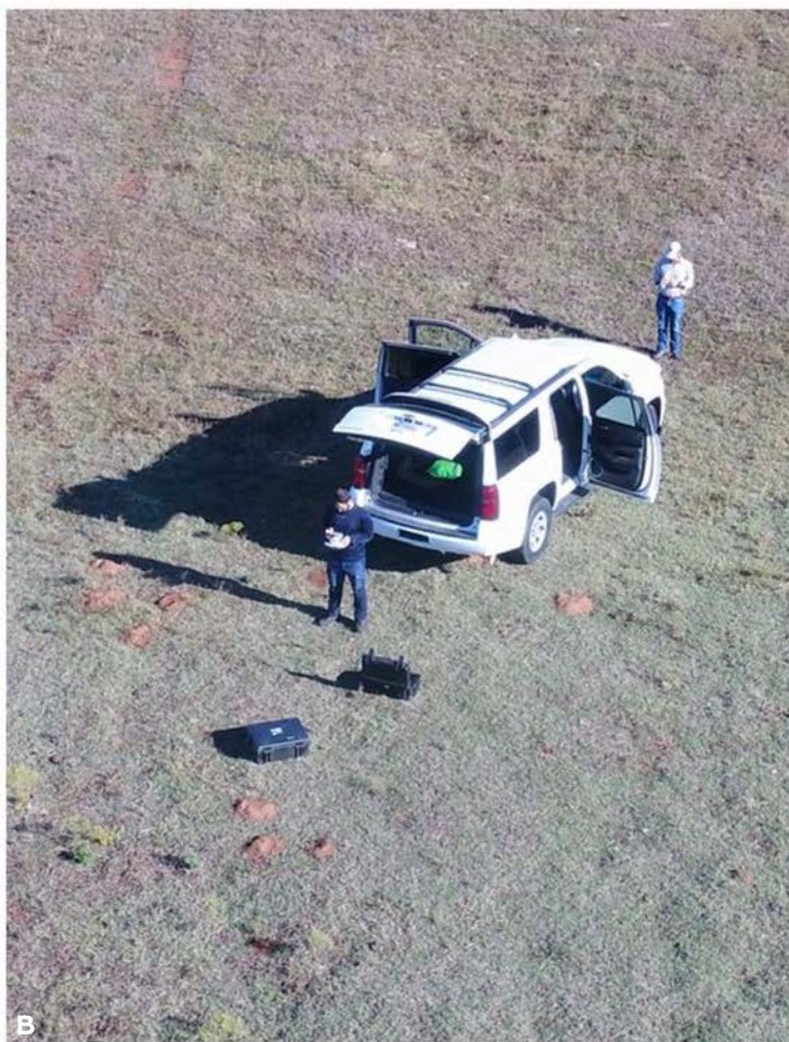
Figure 1 – A: The complete setup of the magnetic survey installed on a small drone (The non-metallic sleeve carries the smartphone which is mounted below the drone with a 1.5 m non-magnetic cable). B and C: Operating the drone. D: the exposed wellhead.
