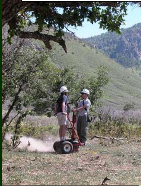
Above: Student Dustin Sweet firing the Betsy Gun during seismic data acquisition across the canyon.
