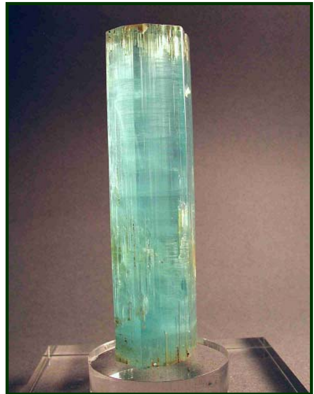
Aquamarine (variety of beryl), Gilgit, Pakistan. This doubly terminated 12-cm crystal contains crossing planes of fluid inclusions that give the crystal a layered, “parfait” appearance. (David London specimen and photo)
