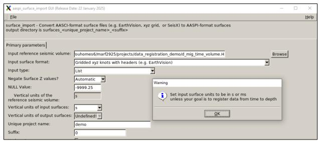
Note that the *Vertical units of the reference seismic volume* is filled in as "s" and cannot be altered. These are the units of your input data volume. In all cases except when converting time to depth or depth to time in AASPI program **surface\_driven\_data\_registration**, these will also be the vertical units of your output AASPI-format surfaces.
