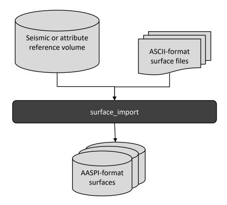
The flow chart is simple. The input files include an AASPI-format ("\*.H") file that represents the extent of the seismic survey as well as one or more ASCII-format ("text") files of the same type exported from an interpretation workstation or geostatistics program. The output consists of a corresponding suite of AASPI-format surface files that are either truncated or extended (using null values) corresponding to the input reference seismic data or attribute volume.
