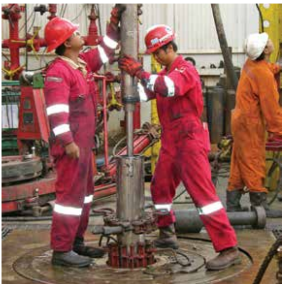
Figure 2. My teammate and I (red coverall in the middle) were assembling special tools to drill an oil well and gather subsurface data in offshore Strait of Malacca, Indonesia.
