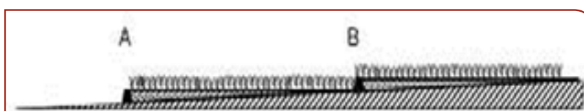
Figure 13.20: A series of continuous bed stabilisation structures on a gully floor
