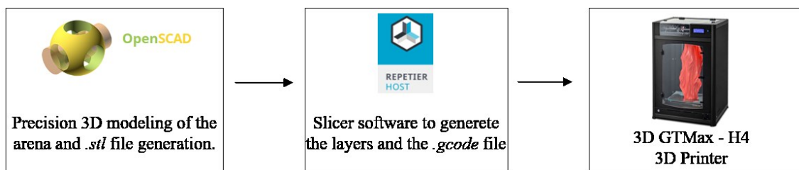
Figure 1. Process for printing the lane-maze.
