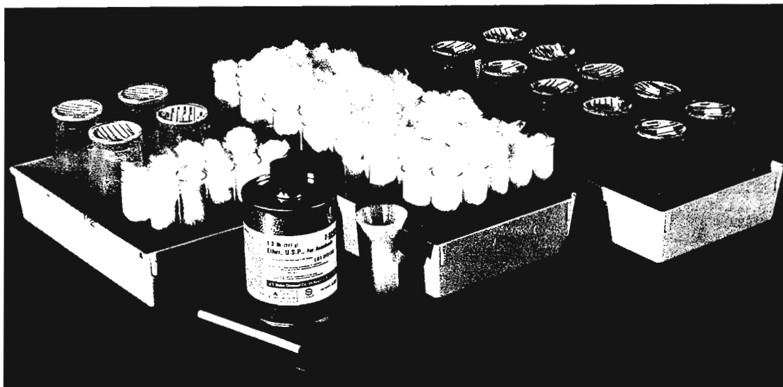
Fig. 3. Bottle and vial trays and ether anesthetizer used for Drosophila rearing.
