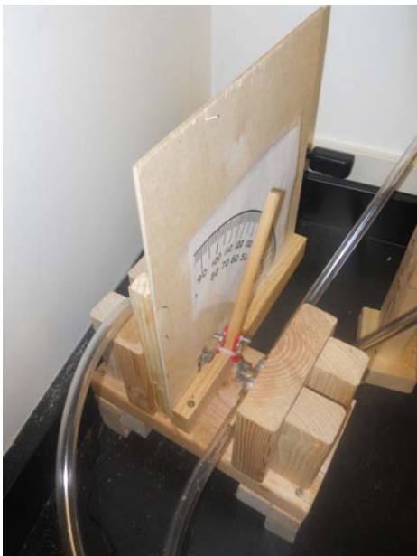
Figure 3. The dose selector was built from construction grade lumber and plywood. Two 3/8" ball valves are mounted orthogonally to each other to form a constant output diverter valve. The red handles of these valves are visible in this image. The wooden dowel was secured to both handles with two bolts and a zip tie.
