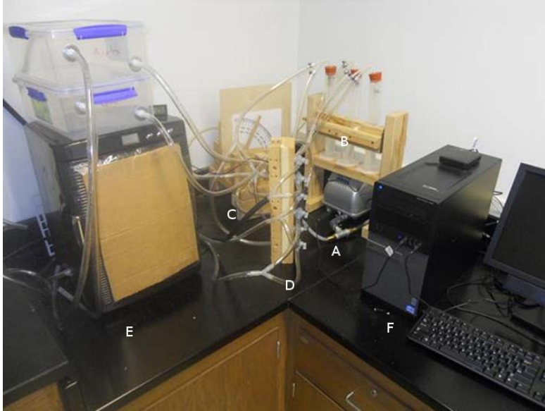
Figure 1. The ethanol delivery system and locomotor activity apparatus. A, air pump; B, gas washing bottles; C, dose selector; D, valve bank; E, incubator; F, computer. Details of each component are provided in the text and other Figures.
