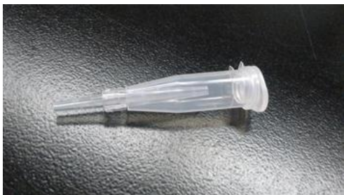
Figure 1. The olfactory trap apparatus. Flies enter the trap in response to olfactory cues originating from an odorant placed in the cap.
